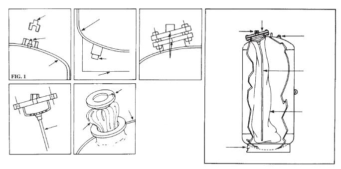
Do not remove the drain plug or loosen the nuts on the blind flange or system connection.
