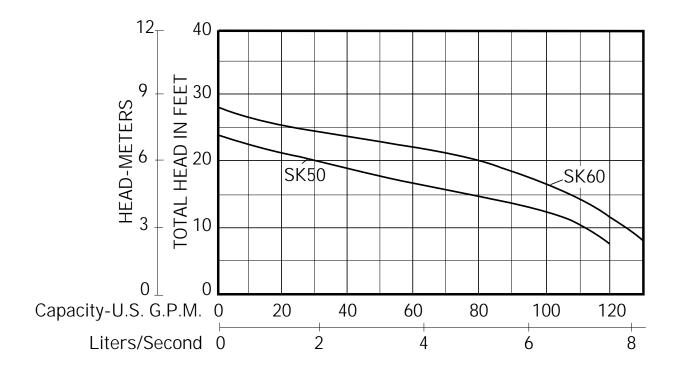
The curves reflect maximum performance characteristics without exceeding full load (Nameplate) horsepower. All pumps have a service factor of 1.2. Operation is recommended in the bounded area with operational point within the curve limit. Performance curves are based on actual tests with clear water at 70° F. and 1280 feet site elevation.
