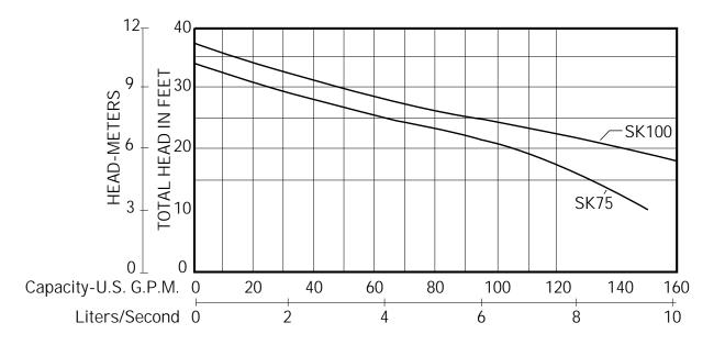
The curves reflect maximum performance characteristics without exceeding full load (Nameplate) horsepower. All pumps have a service factor of 1.2. Operation is recommended in the bounded area with operational point within the curve limit. Performance curves are based on actual tests with clear water at 70° F. and 1280 feet site elevation.
