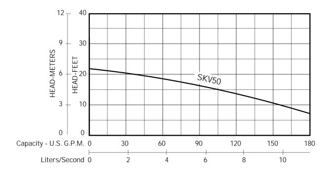
The curves reflect maximum performance characteristics without exceeding full load (Nameplate) horsepower. All pumps have a service factor of 1.2. Operation is recommended in the bounded area with operational point within the curve limit. Performance curves are based on actual tests with clear water at 70° F. and 1280 feet site elevation.
